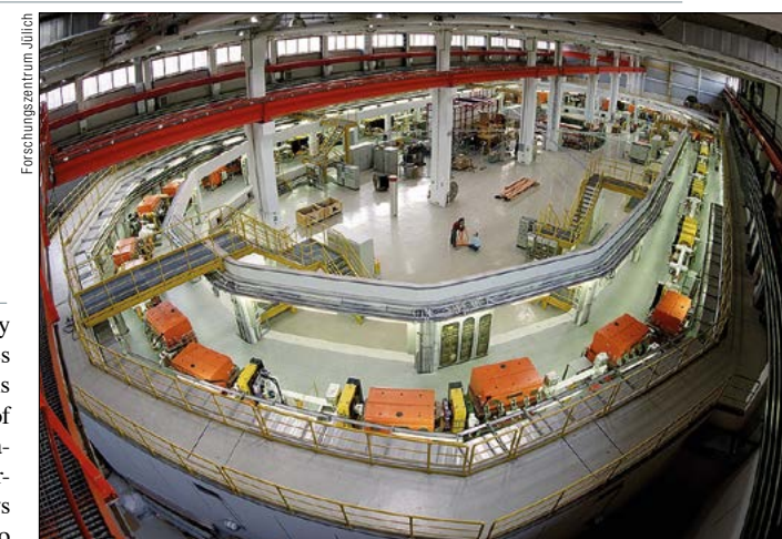
The COSY storage ring at the Forschungszentrum Jülich in Germany is being modified to search for very small electric dipole moments.
