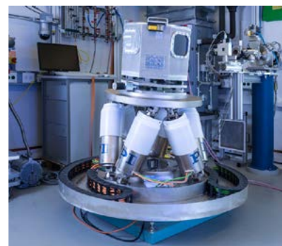
Fig 3: Hexapod in the experimentation station EH3 on the P07 beam guidance unit on PETRA III: With its high load capacity, it can carry the entire measuring setup including the structure where mechanical forces are applied – in this figure a chamber for the laser-welding of titanium aluminides. (image: PI / HZG)
