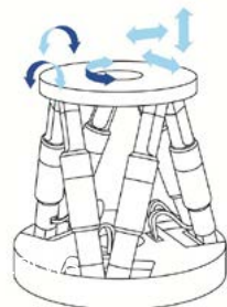
Fig 2: Basic design: In parallel-kinematic systems, all actuators act directly on the same platform. (image: PI)
