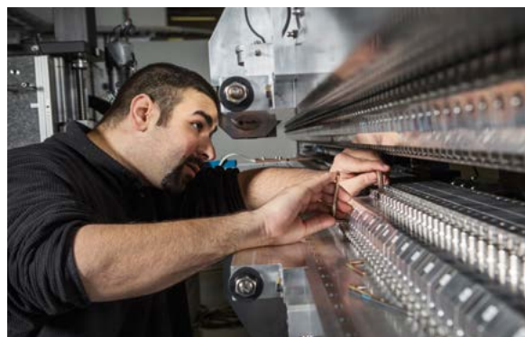
An undulator at MAX IV, which generates intense synchrotron X-rays as electrons pass through a periodic magnetic structure.
